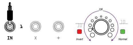
With nothing patched into any of the inputs the control knob will simply output a static voltage. The control knob will adjust the static voltage level and polarity in this scenario
