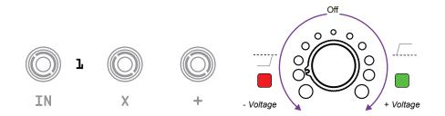
When a signal is patched only into the sum input, the knob will act as an offset. This allows us to shift the input signal in a positive or negative direction without changing the amplitude or polarity of the signal. When a signal is also patched into either the main or multiply inputs any signal patched into the sum input will be added to the results of the attenuverter voltage processor.
